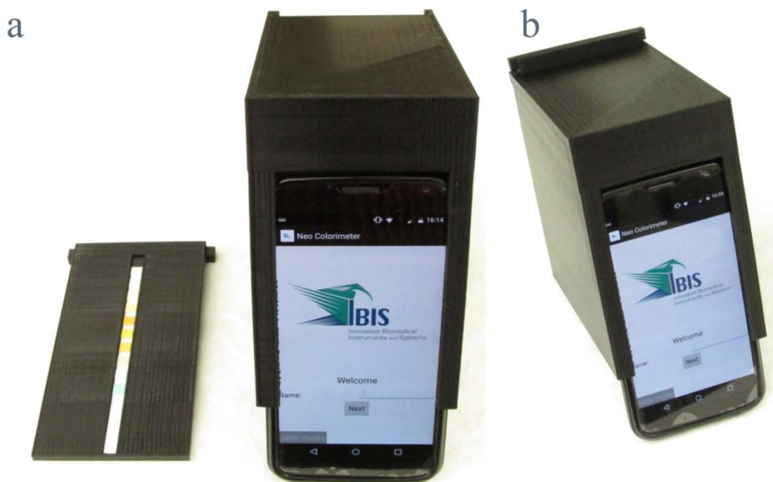
Figure 2.3. (a) Mobile phone based colorimeter with a cassette and a holder, (b) the cassette is inserted.
